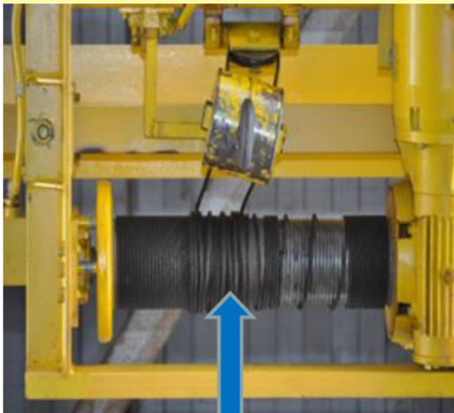
Improperly spooled hoist drum / miss-spool
